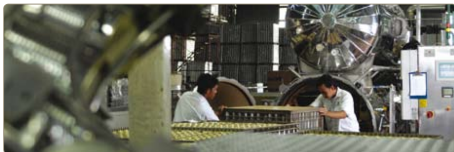
Dairies Division: Steriliser for evaporated milk
